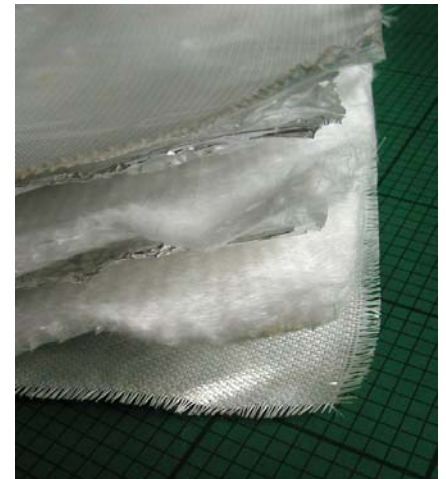
3 foil layers interleaved with high temperature glass fibre construction
